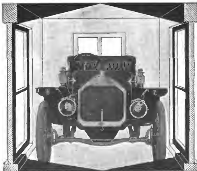
Fig 4—A narrow structure with the windows passing down almost to the floor line and lighting up the machinery portion of the automobile
